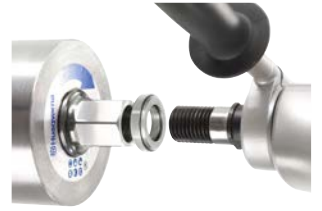
4 Washer quick release, to release the drill motor thread from the drill bit
